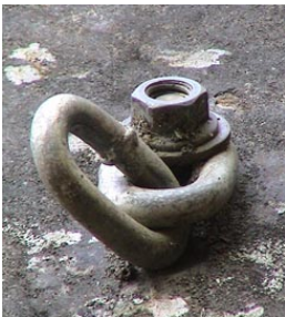
Captive chain where nut has limited thread. Chains links used this way can place large outward forces on the bolt.
